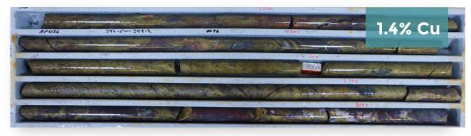
AP034 high-grade Cu mineralization (chalcopyrite) in 1m interval (189-190m) grading **3.1% Cu** within: **5m** @ **2.06% Cu** from 187m (within wider zone: 31.6m @ 0.64% Cu from 177.7m)
