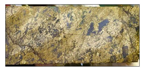
Photo of drill core from SDD005 (353.5m), showing high-grade IOCG style pyrite-chalcopyrite-bornite magnetite mineralization (353-354m: 1.3% Cu, 0.49g/t Au).
